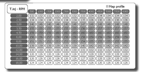
This menu shows a numerical display of the multiplication coefficients called K the control unit uses in calculating the GAS injection time.
